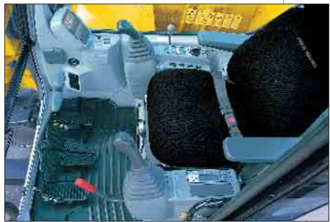
**"High Space"** cab with perfect visibility in all directions thanks to the wide glass area and transparent cab roof. Extremely low noise level and effective reduction of vibrations.
