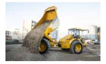
MultiTip makes several working situations easier. For example when tipping a certain amount of payload sideways, whilst moving forward.
