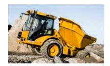
A well proven 6 speed ZF Soft-Shift transmission offers full auto or manual shift. This intelligent transmission will automatically shift 2 gears in the right conditions to smoothly increase acceleration regardless of the payload.
