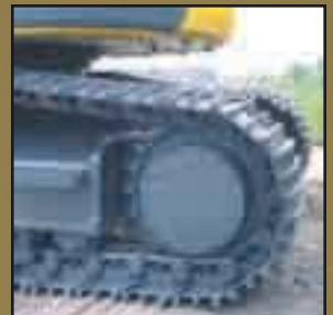
Larger sized travel motors and heavy duty undercarriage enhance durability.
