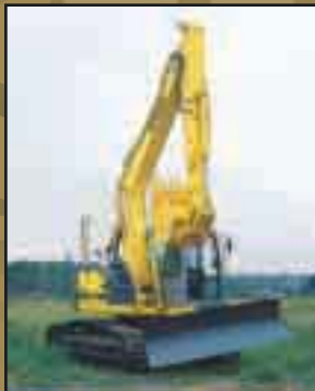
The ED150 comes standard with a Power Angle Tilt (P.A.T.) blade with a 2.86 cu yd capacity.
