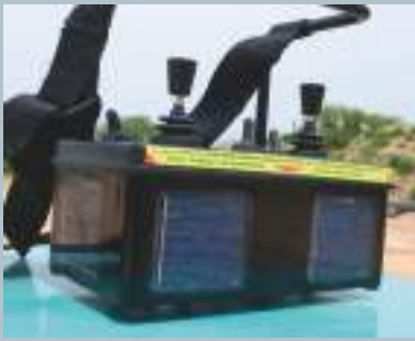
IR transmitter with solar panels
