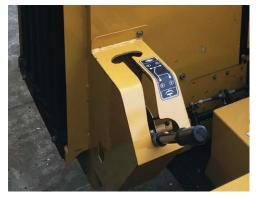
**CLUTCHLESS PTO SYSTEM.** A clutchless PTO system allows the cutter to be engaged without using a traditional slip clutch or idler pulley and without sliding the engine.
