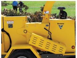
MINIMISE MAINTENANCE. Once the shield is opened, belts can be changed without tools, and the clutchless PTO system eliminates the need to slide the engine.
