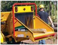
**OPERATOR SAFETY.** With the patented bottom feed stop bar, the four-position upper feed control bar with dual stop positions and forward / reverse feed positions mounts over the feed table.
