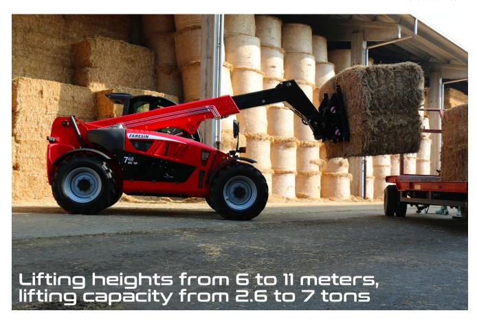
The telescopic boom is made of **Domex \$420 steel** it is hinged in the chassis at a lowered position: this assures maximum visibility during loading operations and a better weight distribution.
